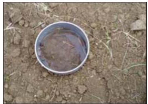
Figure 166. Water draining into soil. Credit: USDA, Soil Health Testing Kit Guide, August 1999, https://efotg.sc.egov.usda.gov/references/public/WI/Soil_Quality_Test_Kit_Guide.pdf
