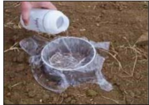
Figure 14. Adding water. Credit: USDA, Soil Health Testing Kit Guide, August 1999, https://efotg.sc.egov.usda.gov/references/public/WI/Soil_Quality_Test_Kit_Guide.pdf
