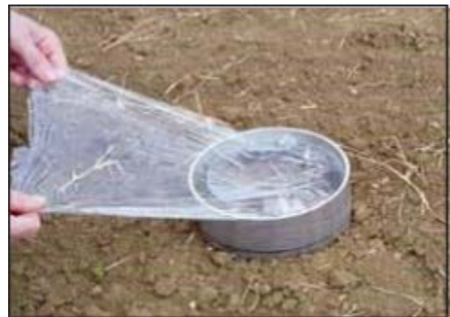
Figure 155. Removing plastic wrap. Credit: USDA, Soil Health Testing Kit Guide, August 1999, https://efotg.sc.egov.usda.gov/references/public/WI/Soil_Quality_Test_Kit_Guide.pdf
