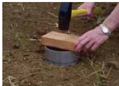
Figure 13. Driving ring into soil. Credit: USDA, Soil Health Testing Kit Guide, August 1999, https://efotg.sc.egov.usda.gov/references/public/WI/Soil_Quality_Test_Kit_Guide.pdf
