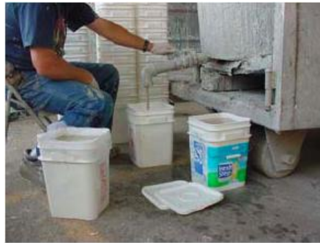
Figure 7: Paint is mixed and poured into buckets. Source: 16.
