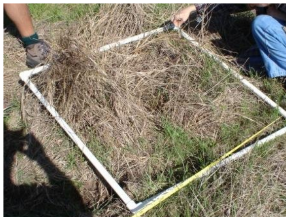
Figure 7: Example of a 1m 2 quadrat used to estimate floristic abundance via “percent cover”. Quadrats were deployed across a 10m transect. Source: Sampling Vegetation Attributes, Bureau of Land Management (1999).
