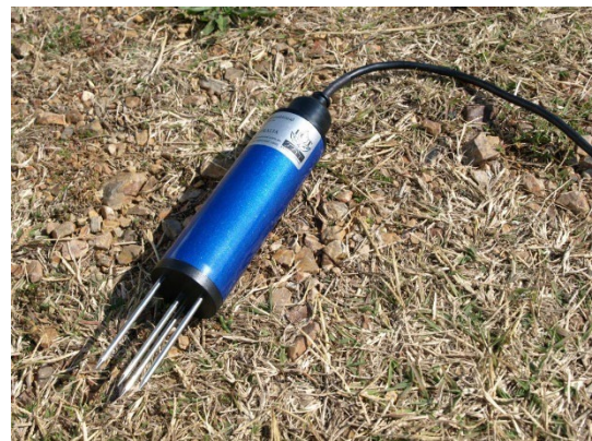
Figure 4: Soil moisture probe. Source: ICT International ( https://ictinternational.com/product/mp406-soil-moisture-sensor/ )
