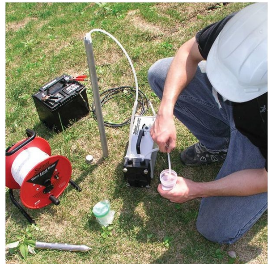
Figure 6: Water level sensor being deployed into a catch basin to measure a site's water table height, depth, and flow direction. Source: Solinst ( https://www.solinst.com/instruments/level-measurement-devices/ )
