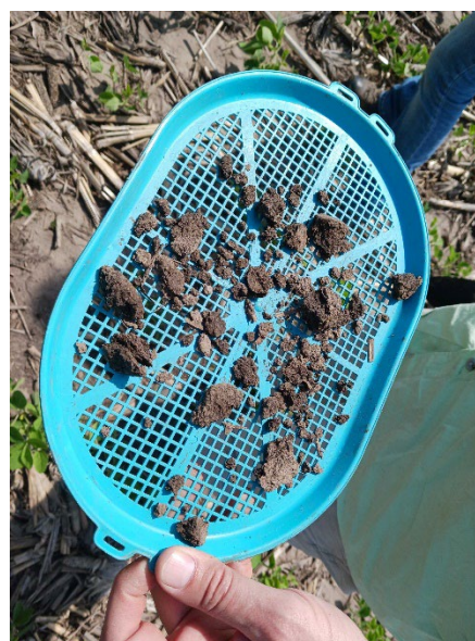
Figure 7: Collection of pea-sized aggregates to fill a 50 mL centrifuge tube from the top 3" of soil for soil aggregate analysis. Source: Delta Institute
